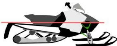
It is ideal to have a balanced vehicle with the suspension's ride height set at 1/3 the overall travel in both the front and rear.
